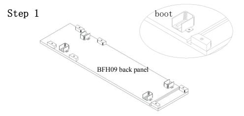
Slide boot is installed on the BFH09 back panel
